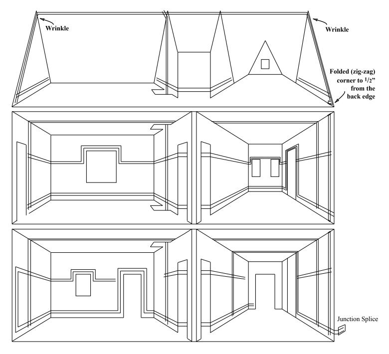
The run thru the Electrification Slots was made from the top down (a craft knife is needed to coax the tapewire thru the E-Slot on the Top Floor), then a folded corner just above the floor on the Attic Endwall brings the tapewire to 1/2° from the the back edge and changes angle without needing a connection (which would interfere with the connection to the attic
