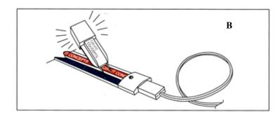
Proceed to the 2<sup>nd</sup> floor and begin your run on one end of the house. No need to wrap the tape onto the outside of your house on the 2<sup>nd</sup> or 3<sup>rd</sup> floor. When you reach the end of the last wall on the 2<sup>nd</sup> floor, cut the tapewire. Continue the process on the 3<sup>rd</sup> floor as well.
