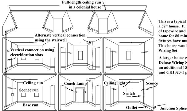
This is a typical tapewire layout for a 32" house. It uses about 42 feet of tapewire and might become the home for 80 miniature bulbs (many fixtures have multiple bulbs). This house would use the Deluxe Wiring Set
