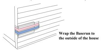
The first obstacle will be the front door. Rather than cutting the tape, fold the corners for a continuous run.
