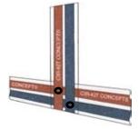
**The Ceiling Run**: Begin at the base run of the desired room and run up the wall and across the ceiling. Attach this new run to the baserun with 2 eyelets. An adapter will be used to attach the ceiling light to the tapewire at a later time. Lightly spackle and paint or cover with a ceiling paper.
