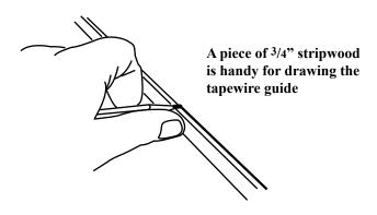
Once pencil lines are drawn, begin to lay the tapewire. Choose a starting point on either end of the house. Start by wrapping 3" of tapewire on the outside of the house, and then proceed to run the tapewire just above the pencil line. It does not matter which color is on the bottom or top. Follow the pencil line using the doorways to move from room to room.
