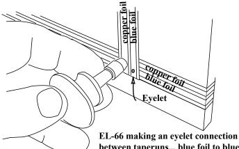
between taperuns... blue foil to blue foil, and copper foil to copper foil Now is a perfect time to test the tape wire on each floor. Use your tester at the beginning and end of each tape run. Make sure that your tester lights up. If nothing lights up, check your transformer, lead in wire switch, and Junction Splice. If you do have power *before* a connection but do not *after* the connection, add a brad or eyelet to each color foil at that connedtion.
